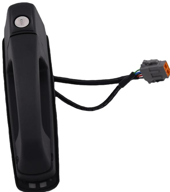
TriMark's new 020-0870 e-LOCK Pull Handle for off-road applications, allows use with TriMark's Gen 3 e-ASK Passive Keyless Entry System featuring integrated capacitive sensor, PKE circuit board and power lock/unlocking motor drive. Based on the proven 020-0850, this robust pull handle brings the latest automotive functionality and convenience to your cab enclosures.
